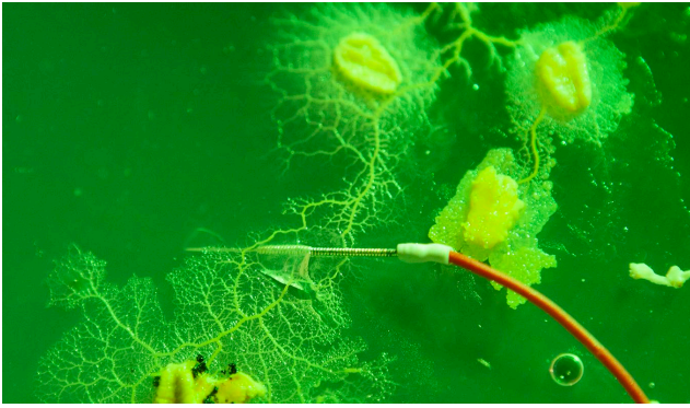
Figure 11: Silver electrode needles used to induce bio-electrical conduction and subsequent resistance measurements. ©somme.
